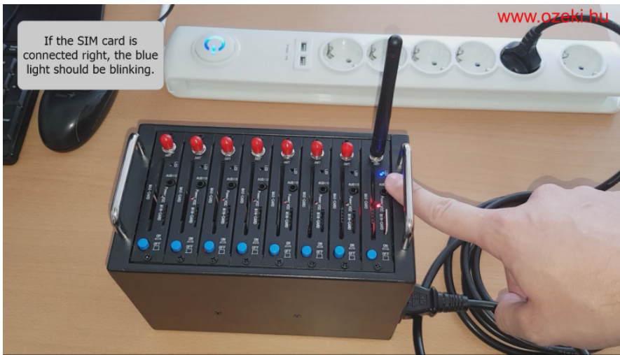
Figure 6 - The blue light indicates the status of connectivity
