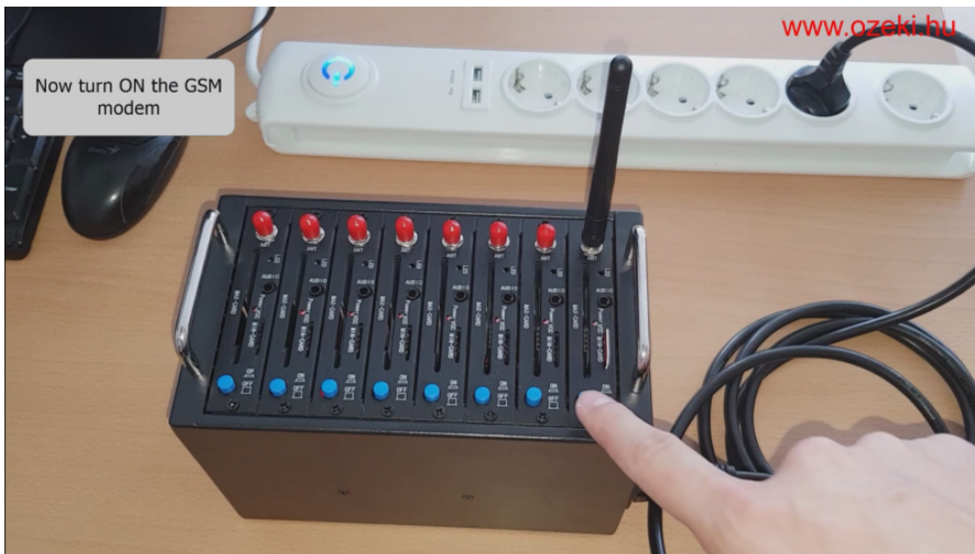
Figure 5 - The ports can be turned on or off separately
