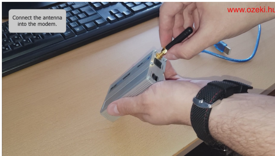
Figure 3 - The antenna connected to the modem
