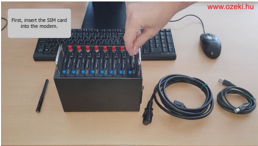
Figure 1 - Insert the SIM card
