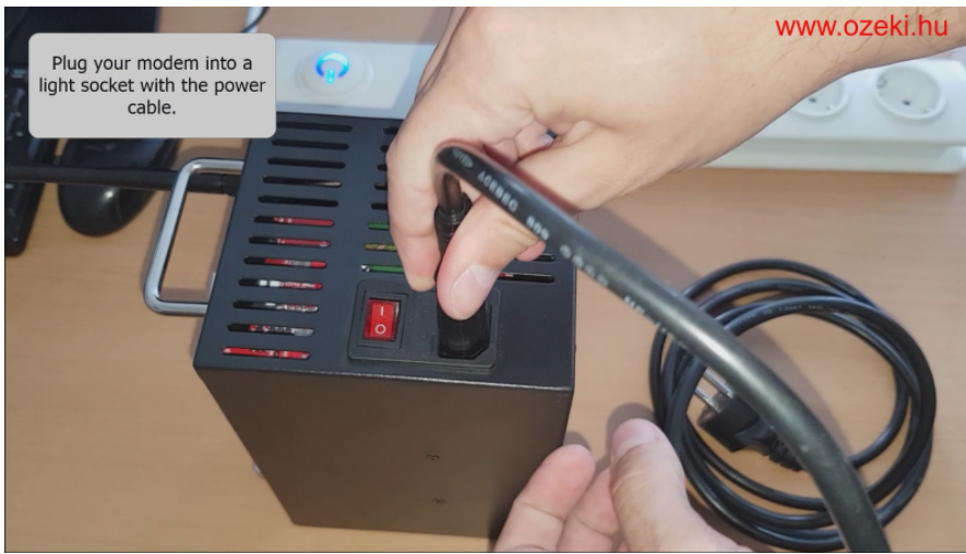
Figure 3 - The power cable plugged into the modem pool
