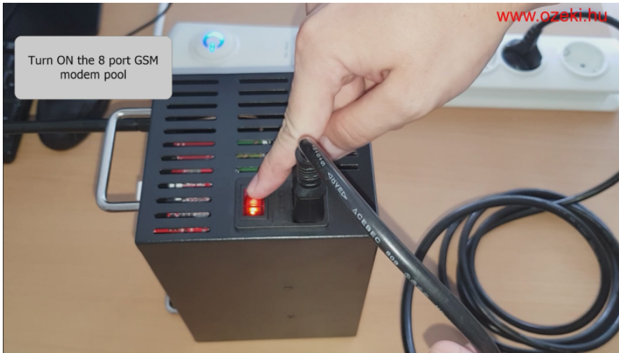
Figure 4 - The modem pool is now turned on
