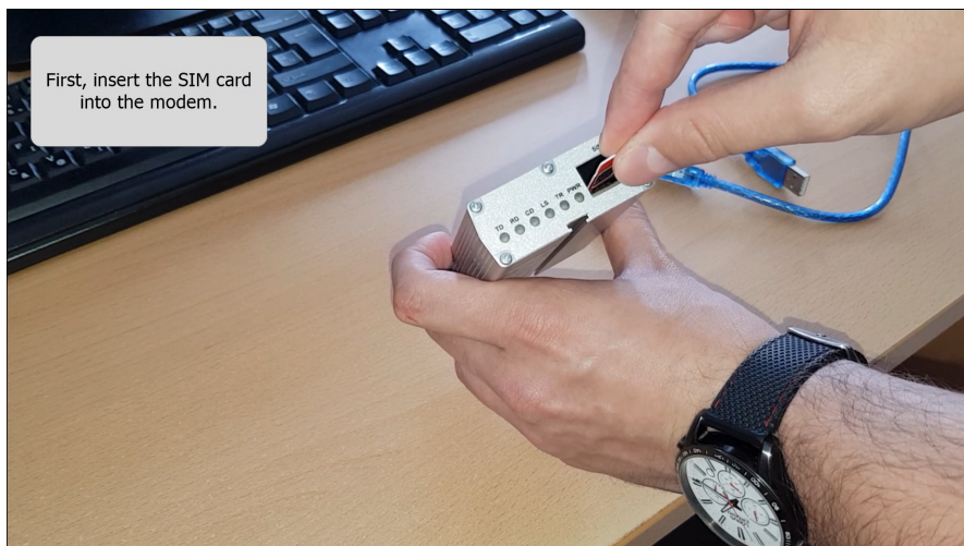
Figure 2 - The SIM card inserted into the modem
