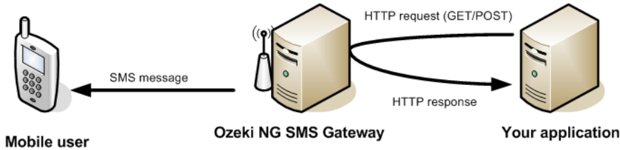
Figure 1 - Send an SMS messages through the built in webserver
